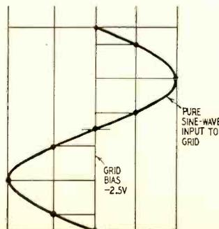
Fig. 6—Using load line information to determine amount of distortion.
