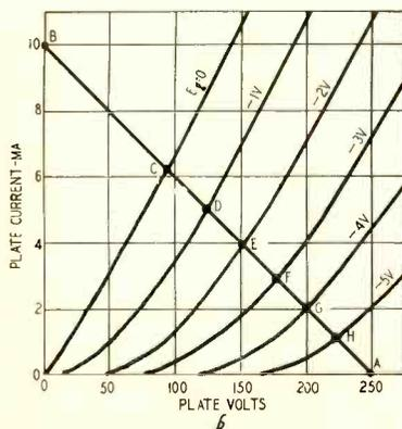
Fig. 5—Showing load line principle.
